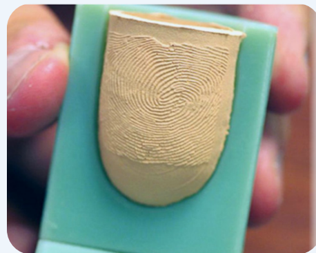
A fake fingerprint spool created at Michigan State University to test fingerprint scanners. Image Credit: Michigan State University.
